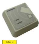
UW-DAL is RFID reader module working on the principle of contactless reading data from Unique transponder (EM MICROELECTRONIC MARIN SA - P4150). Unique transponder has "Read Only" memory with 40-bit identification number stored in it ( ID numbers are different for each transponder). Reader sends this number via 1-wire Bus in format DS1990.
