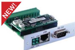
With the PI module made by AK-NORD, a subsequent connection of serial terminals to LAN, ISDN or Bluetooth can be easily performed. The RS232/V24 or an internal RS485 interface are offered in the device. Only a small outlet of 64 x 20mm is required in order to plug the PI modules in the terminals. The PI modules are fixed with two screws and internally supplied with a tension of 6 to 40 volts.
