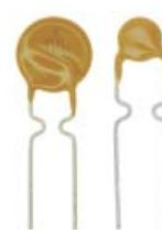
PolySwitch devices are polymeric positive temperature coefficient (PPTC) devices, which are used to help protect against harmful overcurrent surges and overtemperature faults. Like traditional fuses, these devices limit the flow of dangerously high current during fault conditions. However, the PolySwitch device resets after the fault is cleared and power to the circuit is removed, thereby reducing warranty, service and repair costs.
