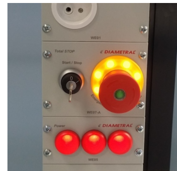
Power control of the table with switch, signalization and illuminated TOTAL STOP button.
